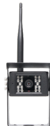
RVS-55W SimpleSight™ 130° Wireless Backup Camera With 18 Infra-Red Illuminators
